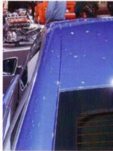
Laser brazed solution without plastic roof trim
